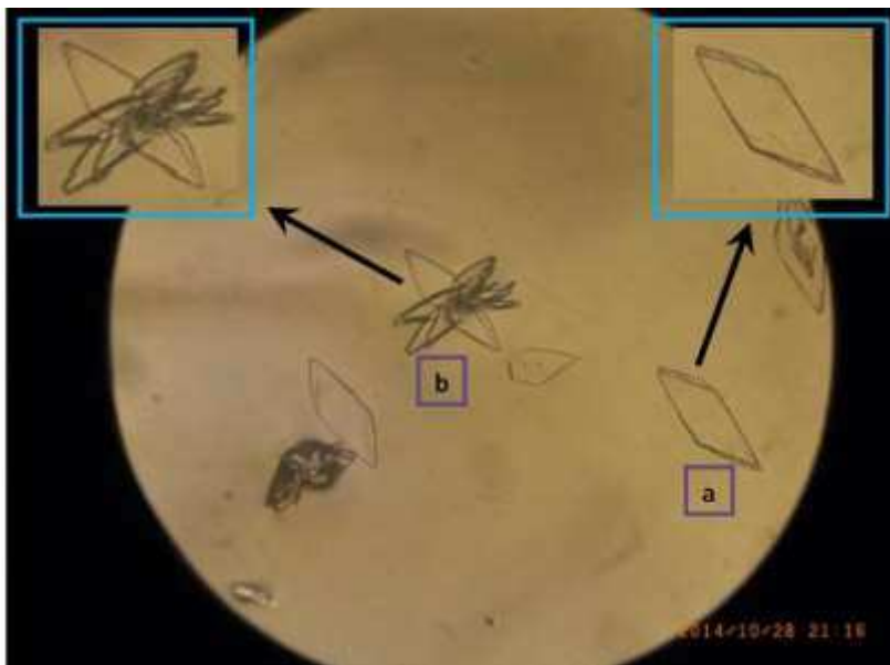
Figure 1.3: Formation of CHPD crystals. a. tetragonal bipyramidal ; b. star shape.
