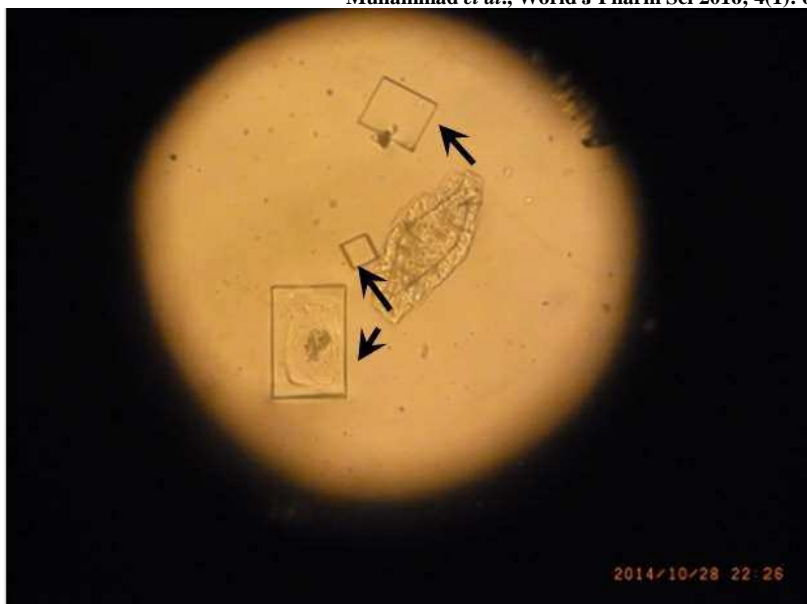
Figure 1.4: Conversion of CHPD tetragonal bipyramidal crystals into COM cubical crystals.
