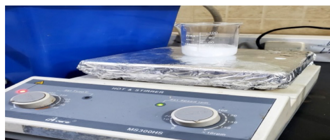
Figure 1: The process of dissolving poloxamer 407 (P407) using a hot stirrer plate.
