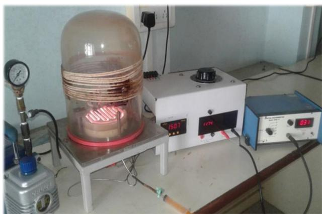
Fig. 3. Photograph of steady gas sensing system.
