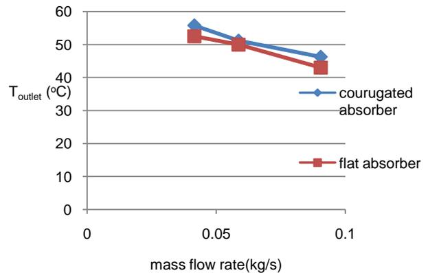
Fig. 12 Variation of outlet temperature with mass flow rate
