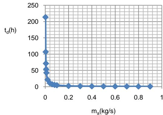
Fig. 3 Drying time variation with mass flow rate of air at fixed coffee mass (20kg) and dryer inlet temperature (38°)
