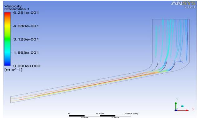
Fig. 9 Velocity streamline for smooth curve connection with guide vanes
