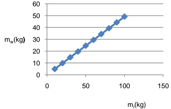
Fig. 2 The variation of moisture to be removed vs initial coffee mass at fixed initial moisture content ( $MC_{wi}=55\%$ )
