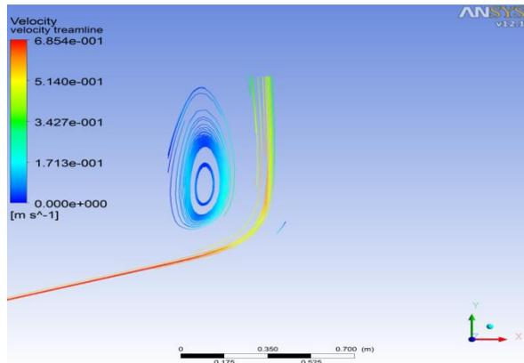
Fig. 6 Velocity streamline for sharp edge connected configuration
