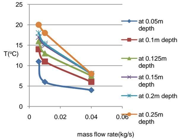
Fig. 11 Temperature rise of air at different collector depths
