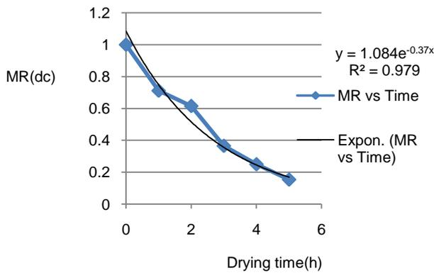
Fig. 14 Variation of moisture ratio against drying time for clear sunshine day and the curve fit
