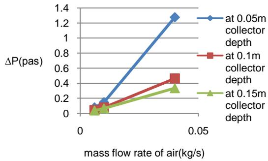
Fig. 5 System Pressure drop variation with collector depth at different mass flow rate of air
