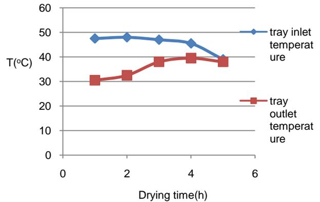
Fig. 13 Variation of drying tray inlet and outlet temperatures during drying time for clear sunshine day
