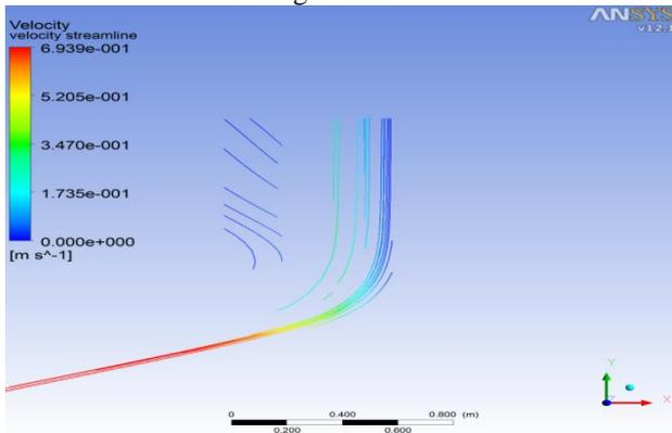
Fig.7 Velocity streamline for smooth edge connected dryer Configuration
