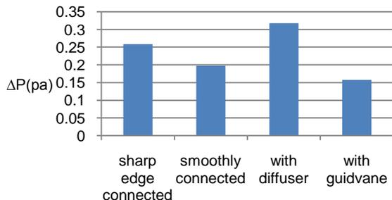
Fig.10 Comparison different geometry for pressure drop
