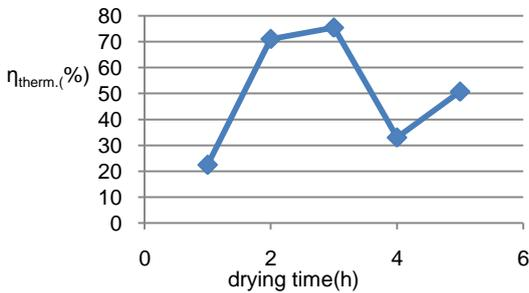
Fig. 15 Variation of thermal efficiency of dryer during drying time for clear sunshine day during experimental testing
